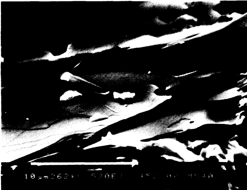
Fig. 5. SEM photograph of the broken surface of a BPSCCO-AG sample annealed for 40 h. The composition of the aggregates on the plates is \text{PbCa}_2\text{O}_4 ,
