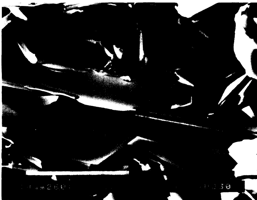
Fig. 6. SEM photograph of the broken surface of a BPSCCO sample annealed for 30 h.
